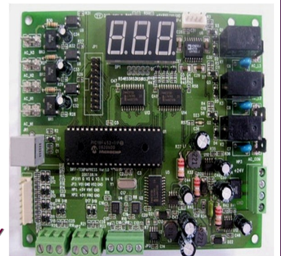
The newly released SC901 Smart Controller for VFD applications.
